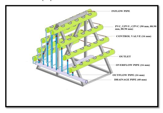
Fig. 1: Isometric view of a shaped frame hydroponic structure
